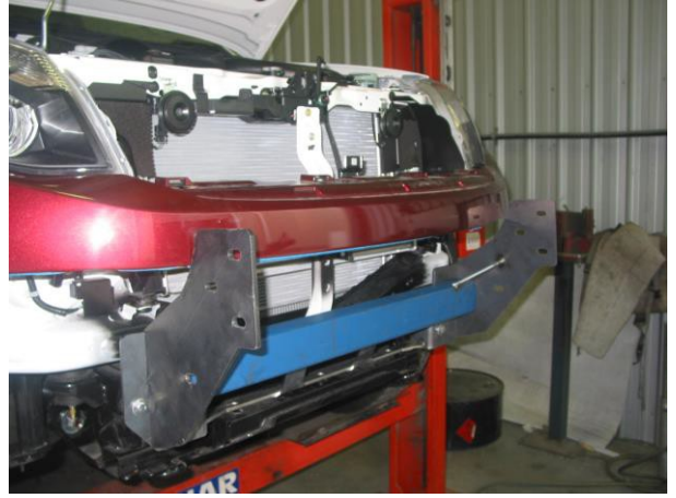
Figure 6: ECB steel mounts with bumper fitted.
