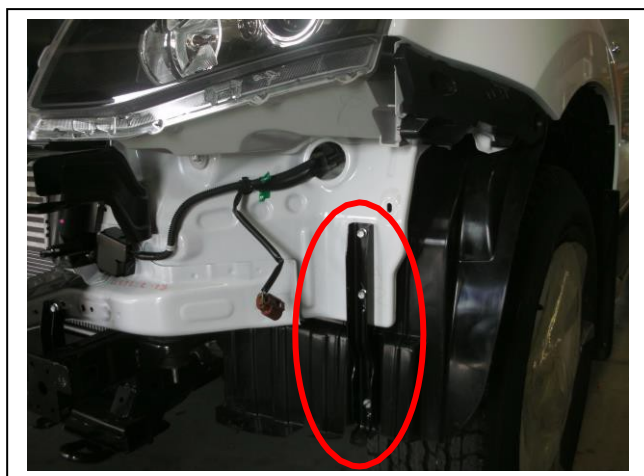
Figure 3: Passengers side outer bumper stiffener
