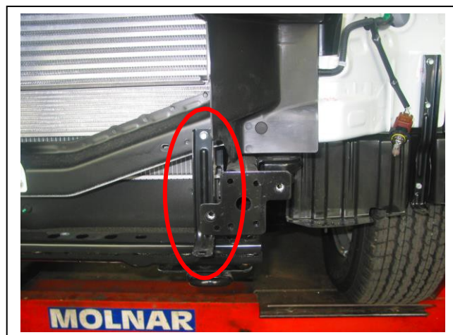
Figure 2: Passengers side inner bumper stiffener
